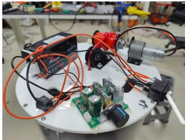
Fig. 9: Integrated Control and Actuation Module with DC Motor, Servo Assembly, and Power Regulation Circuit.
